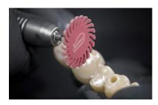
**4.** Pre-polishing of basal surfaces with the red spiral.
